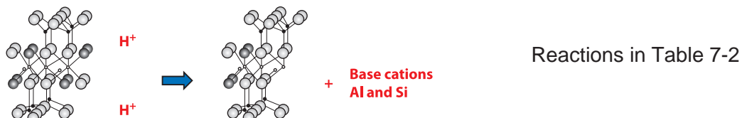
Figure 7-8 Ion-exchange, surface protonation and mineral dissolution serves to consume released acidity.
