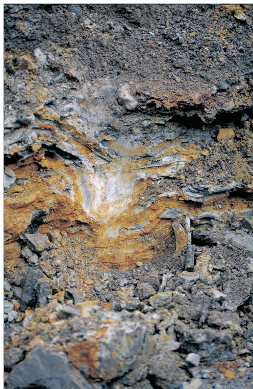
Figure 7-1 Schematic picture of a waste deposit where a soil cover has been applied on previously weathered tailings. Underneath the tailings, a natural soil layer covers the bedrock.
