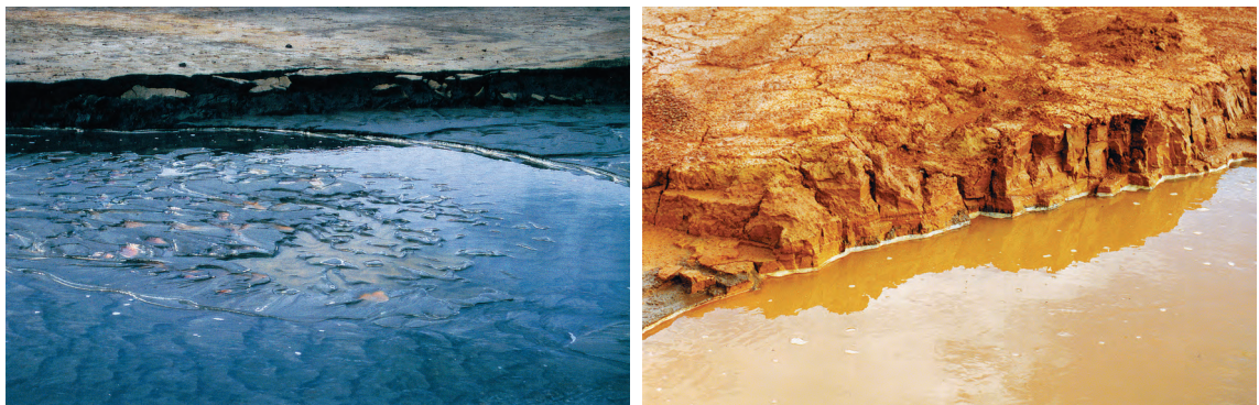
Illustration: Unoxidised tailings to the left and oxidised tailings to the right.
